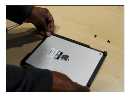
4. With the iPad and the face plate face down, place the base and the back plate over the screw holes and screw in.
