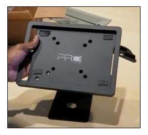
2. Flip the stand over and remove the four screws located on each corner of the back of the Pro Vault enclosure. These must be removed to insert the iPad.
