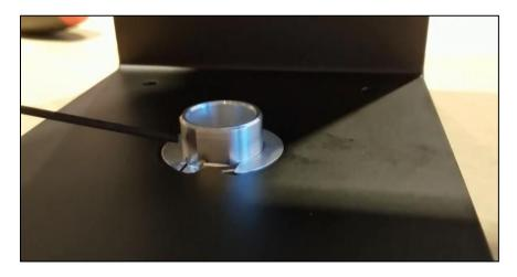
3. Put the cover on with the hole face the flat side of the swivel plate. You can use an adhesive to secure the swivel stand, and you can swivel now.
